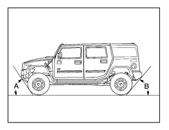
Design specifications required a minimum gradeability of 60% (31°) slope, with the vehicle fully loaded, on high friction surfaces at 6 mph (9.7 km/h).
